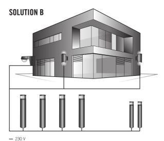
DEFENSOR motion detectors are ideal for controlling ALVA lighting for 230 V. This creates a visually harmonious lighting solution while the safety and control functions of the DEFENSOR series increase building safety even further.
